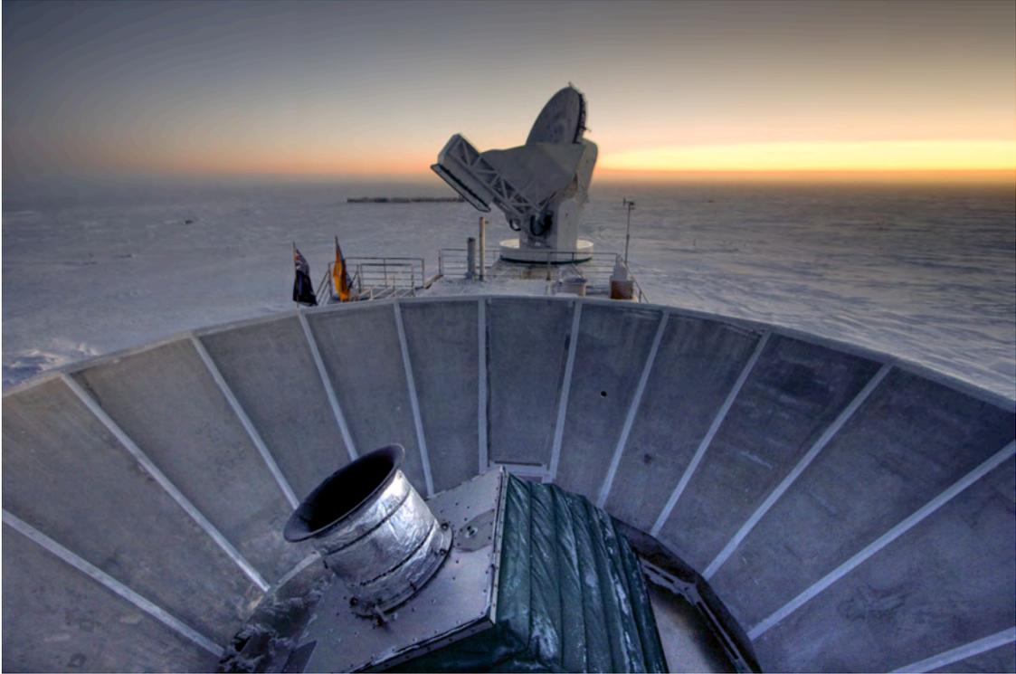
Fig 4. The BICEP prototype polarimeter (foreground) deployed at South Pole station.
