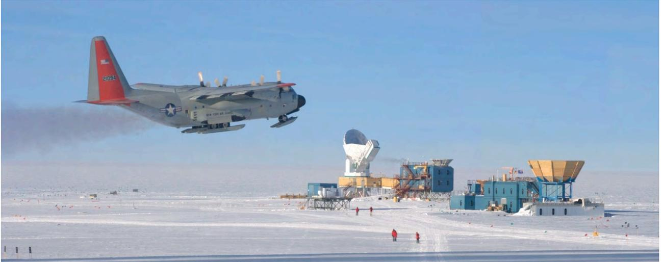
Fig 5. A C-130 cargo plane taking off from South Pole station. Visible behind the runway are the 10 m South Pole telescope (large white dish) the BICEP prototype polarimeter (grey inverted cone on top of blue building) and the mount that will house the Keck Array (wooden inverted cone on far right).
