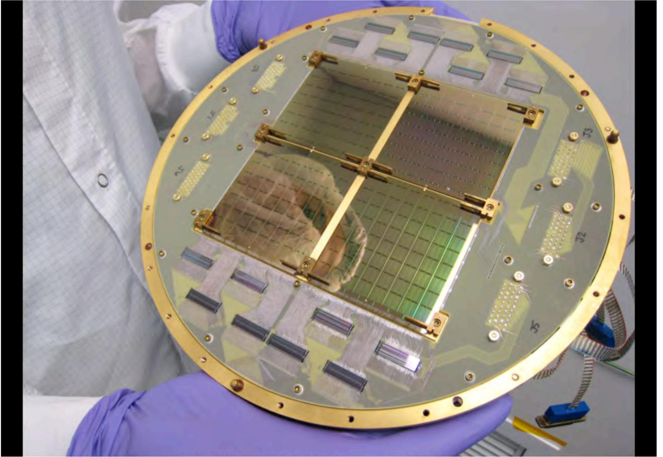
Fig 6. The advanced, polarization-sensitive mm-wave focal plane developed at JPL that will be at the heart of each of the Keck Array polarimeters.
